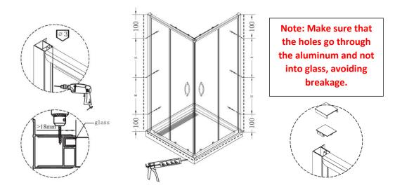
e) Using recommended bathroom purpose silicone. Apply a fine bead of silicone vertically and horizontally on the outside perimeter of screen only, sealing your shower screen. This will prevent water from leaking out of screen and will allow water to effectively drain back towards outlet. Do not use shower for 24 hours allowing for silicone to set.
