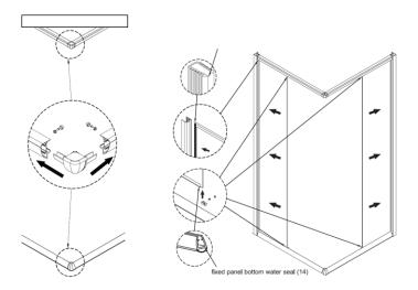
Step 4 Assembly of Door Rollers (Note: You must work out which is top & bottom of both Door panels before applying rollers)
