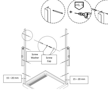
Note: Wall jamb must be Plumb / Level and set in side of tile flange of base or within min and max measurements. Use correct or most suitable fixings for the surface area you are fixing to.
