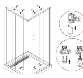
Note: To adjust door; remove roller cover & use Phillips head screw driver. Turn visible screw left or right on top roller allowing the door to lift or lower. Ensure both door hinges are aligned.
