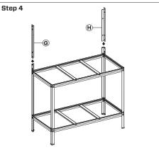
Join the pegboard frame 'G' and 'H' as shown in the diagram. Note upright position.
