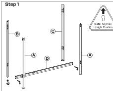
Place foot end caps onto the bottom of the legs 'A', 'B' and 'C'. Note upright position. Place shelving brackets 'D' onto the legs. A rubber mallet can be used to lightly tap all brackets into the keyholes of the legs.
