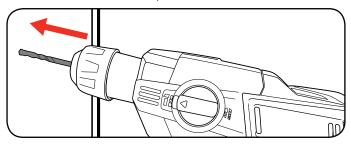
**Note:** Do not force the drill or apply side pressure to elongate the hole. Let the drill do all the work.
