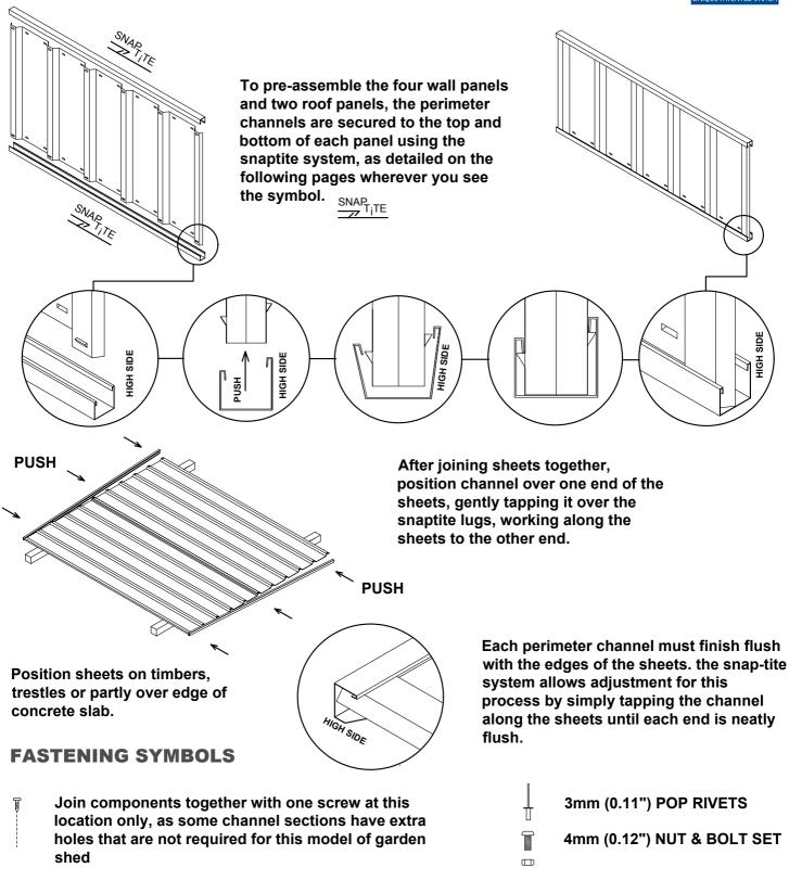
Do not join components together at this location yet, as the screw may obstruct further assembly of other components
