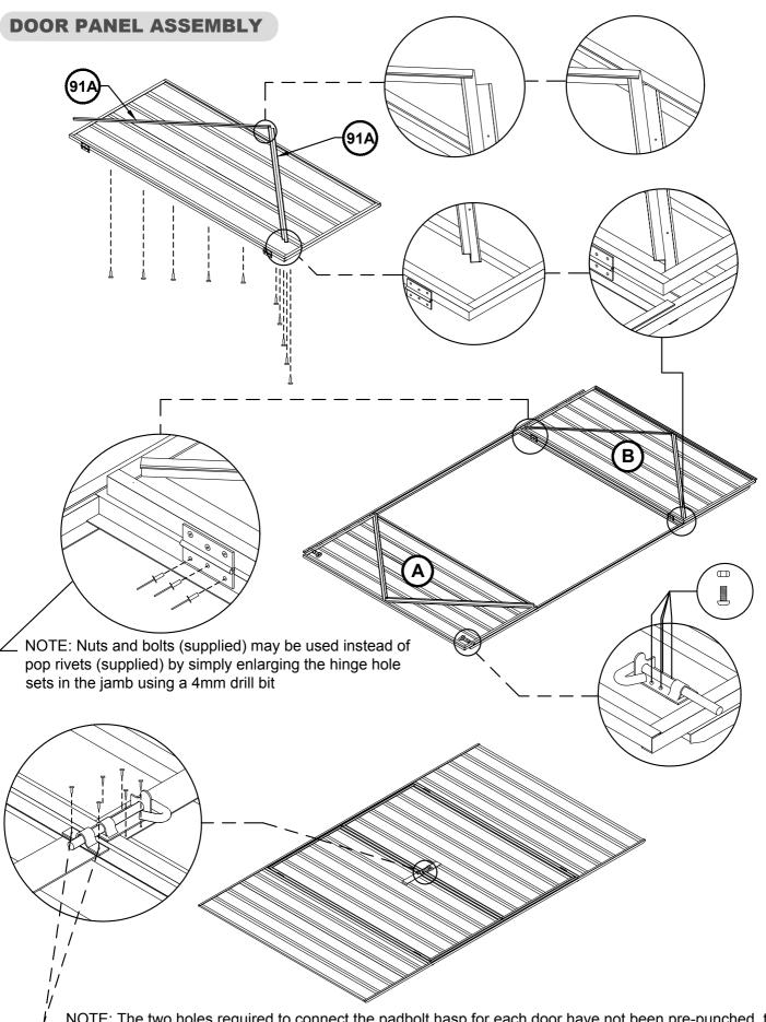
NOTE: The two holes required to connect the padbolt hasp for each door have not been pre-punched, to allow for proper alignment. position each hasp centrally over the padbolt shaft, and drill 3mm holes and secure with screws
