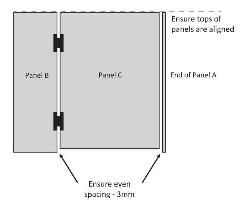
Tighten the hinges and carefully remove the rubber blocks.
