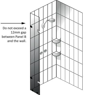
Before tightening all grub screws for Panel B, ensure the door opening is 606mm from the end of Panel A.
