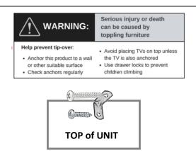
When attaching unit to wall put safety bracket in middle of unit with 16mm pan head screw then 25mm pan head screw into wall. For plasterboard without a stud it is recommended to use a plug with screw (not provided).
