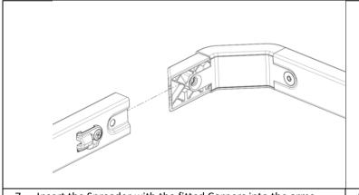
7. Insert the Spreader with the fitted Corners into the arms.
