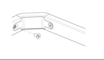
8. Secure each Corner to each Arms using a M6x16mm screw
