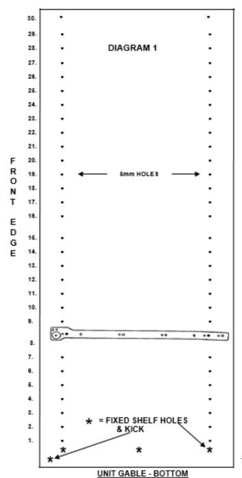
Place metal runners in their correct hole positions (see above) making sure CL = LEFT HAND GABLE & CR = RIGHT HAND GABLE, then attach using the special 7.5mm euro screws provided (see diagram 1)
