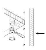
PUSH THE SIDE INTO THE FRONT DOWELS & PIN AND THEN CAREFULLY USING A SCREW DRIVER TURN UNTIL IT LOCKS IN. REPEAT THIS PROCESS WITH THE OTHER SIDE.
