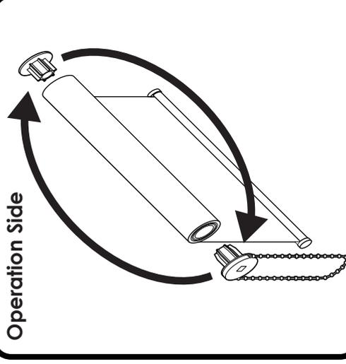
Fabric can be rolled from the front or back by simply flipping the entire roller tube.
