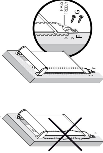
Lightly tension ball chain and fit tension device securely to Architrave/Wall. Allow enough play for chain to pass through device freely.
