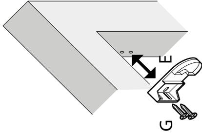
Secure inside window frame as shown above using screws provided
