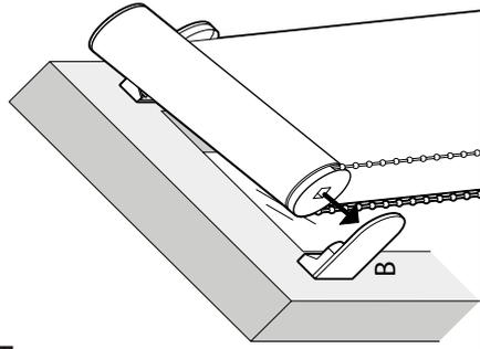
Insert mechanisms into tube on desired sides and insert into brackets.
