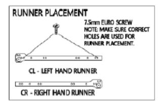
PLACE METAL RUNNERS IN THEIR CORRECT HOLE POSITIONS (SEE ABOVE) MAKING SURE CL = LEFT HAND GABLE + CR = RIGHT HAND GABLE ATTACH USING THE 7.5MM EURO SCREW PROVIDED
