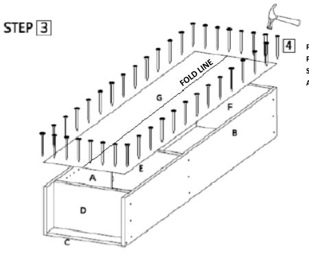
PROCEED TO UN-FOLD YOUR BACK BOARD AND PROCEED TO NAIL IT INTO POSITION MAKING SURE YOU ARE SQUARE AND ON THE EDGE AT ALL TIMES.
