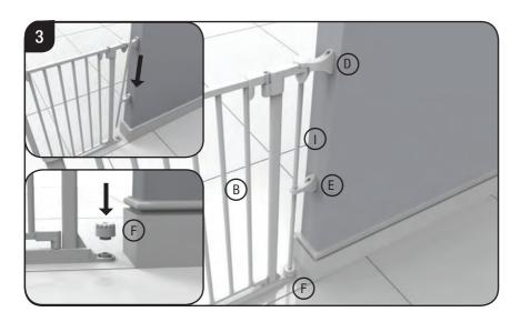
3. Reassemble Panel A, Corner Tube (I) and Top Cap (F) into Top Topside Wall Bracket (D) and Lower Wall Bracket (E).
