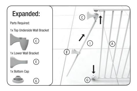
NOTE: Place Lower Wall Bracket (E) over Corner Tube (I) before assembly.
