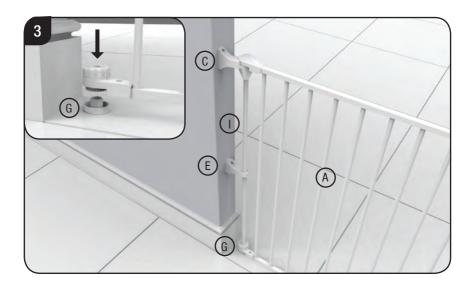
3. Reassemble Panel A, Corner Tube (I) and Bottom Cap (G) into Top Underside Wall Bracket (C) and Lower Wall Bracket (E).
