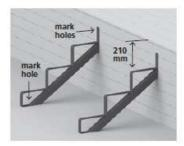
Determine the location of all stringers and ensure the top tread support is 210 mm down from upper deck surface. Then, for each stringer, level and mark the two fastener locations on the deck rim, and one fastener location on the lower deck surface.
