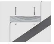
3 Install each timber tread using M8 x 60 mm cup head bolts, nuts and washers.
