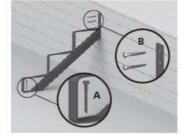
2 A: Attach bottom of each stringer using M10 x 50 mm coach screws\* for timber, or M10 x 60 mm Ramset™ WERCS Ankascrew™ anchors for concrete.
