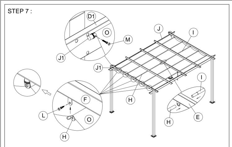
Attach the end fabric hanger (J / J1) to the back connecting bar (D / D1) and fix with bolts M6X30 (M). Attach each elastic loops to end of fabric hangers ( H/I) and fix all fabric hangers ( H/I) to the outer bars (F/F1) by using bolts M6X16 (L). Insert all right fabric hangers (I) to the left fabric hangers ( H/I) through the center bar (E) and into each other.
