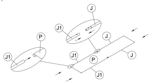
Insert the end right fabric hanger (J) and end left fabric hanger (J1) into each side of sun shelter (P). Make sure J and J1 are inserted to each other.
