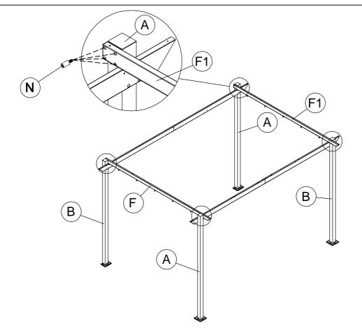
Attach outer left bar (F) and outer right bar (F1) to the post by using bolts M6X15 (N).
