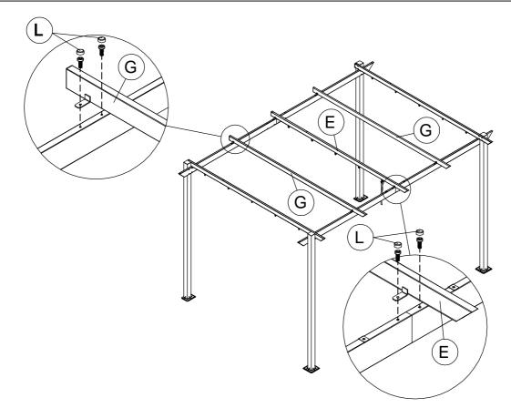
Attach center bar (E) and top bar (G) to the horizontal connecting bar by using bolts M6X16 (L).
