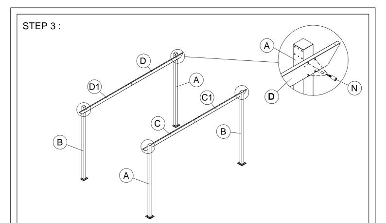
Attach front connector bar (C / C1) to front posts and fix with bolts M6X15 (N). Attach back connector bar (D / D1) to back posts and fix with bolts M6X15 (N).
