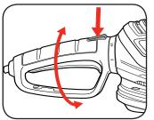
Note: The handle has 5 positions,  $45^{\circ}$  and  $90^{\circ}$  to the left,  $0^{\circ}$  in the centre and  $45^{\circ}$  and  $90^{\circ}$  to the right. The rotating handle button will lock at any of these positions
