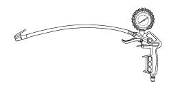
Attach the end of the tire hose to the tire valve. Pull the trigger to increase pressure in the tire as shown on the gauge. To lower the pressure, depress the release valve button.
