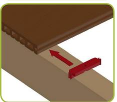
On each joist, insert a fixing clip so that it is positioned within the groove on the decking board and the screw is threaded into the clip only.
