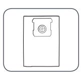
2 To attach, slip the dust bag over the vacuum inlet.
