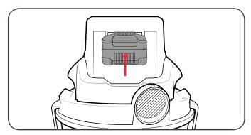
2 To remove, open the battery compartment lid. Press and hold the battery release tab and pull the battery away from the vacuum.
