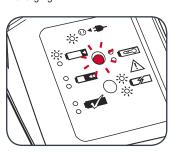
5 The charger LED will illuminate green once the battery is fully charged.
