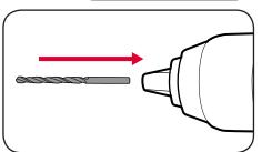
3 Tighten the chuck by turning clockwise.
