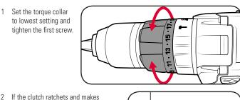
a clicking sound before screw is flush, increase the collar setting and continue tightening.
