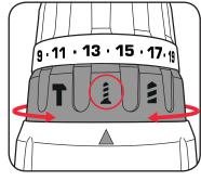
2 To adjust the torque, rotate the torque collar to the desired setting.
