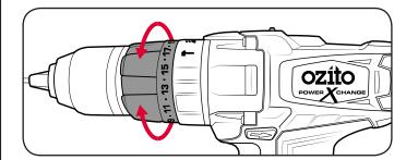
**Note:** Selecting a higher torque setting will allow the drill to use more torque to drive the screw in or out. To prevent damaging the screw head, it is recommended to start at a low torque setting and increase when necessary.
