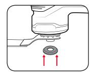
4 Rotate the accessory locking lever clockwise to secure the accessory.
