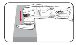
**Note:** Do not apply heavy pressure to the tool or tilt the sanding base as this will wear out the sanding paper and may damage the sanding pad.
