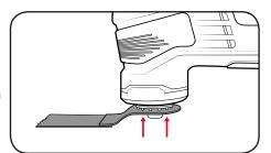
3 When using other non-Ozito multi function tool compatible accessories, the accessory adapter may need to be fitted to secure correctly.
