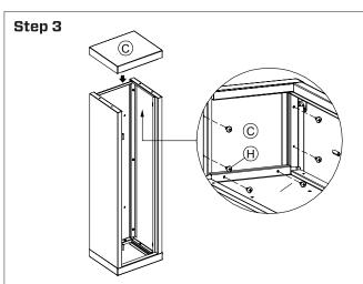
Place remaining side panel (C) onto back (D), top (A) and bottom (B) panels and gently push tabs on the panels neatly into slots on side panel. Once tabs have been inserted, fix all panels together using self tapping screws (H) as per diagram above.
