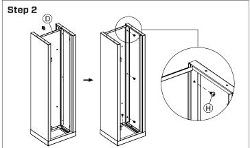
Slide the back panel (D) into side panel (C) ensuring tabs on back panel insert into the slots on the side panel. Then attach back panel (D) to top, bottom and side panels (A, B and C) using self tapping screws (H) as per the diagram above.
