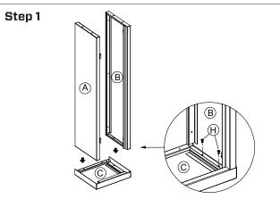
Slide bottom panel (B) into one of the side panels (C) making sure the tabs insert neatly into slots on the bottom panel as per diagram above. Then fix the bottom panel in place using two self tapping screws (H) as per the diagram. Now repeat the same process for the top panel (A).
