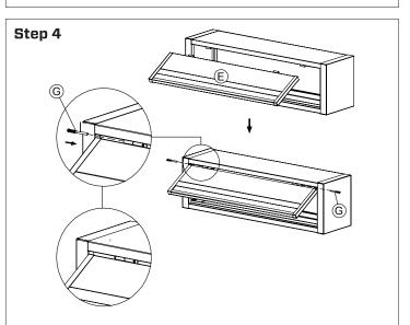
Install door (E) by aligning door hinge slots with those on top panel (A) and insert hinge pins (G).
