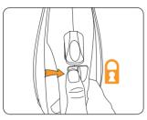
Ensure safety latch is on while the unit is heating.
