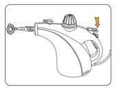
Press steam trigger to release steam.
