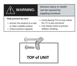
When attaching unit to wall put safety bracket in middle of unit with 16mm pan head screw then 25mm pan head screw into wall. For plasterboard without a stud it is recommended to use a plug with screw (not provided).
