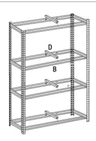
Step 4: Slot Braces (Part D) into position through the holes provided on the Long Beams (Part B).
