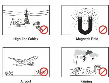
3. Do not fly the APHUBX4 near a magnetic field. There is a compass sensor in the X4 Pro's undercarriage that will need recalibration if it encounters magnetic interference.
