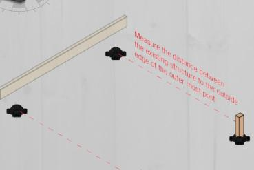
If building off an existing structure, measure from the structure to the outside edge of the post. (For example: If the deck will be 3 metres deep, position the block so that the outside edge of the post is 3 metres from the structure. Do NOT use the the first row of blocks as a measuring reference. Use the same width between the TuffBlock piers as the first row.
