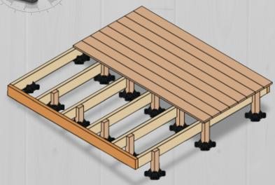
Starting from one side of the deck, attach the first decking board so it's flush to the edge of the deck. The decking board will overhang the first floor joist closest to the existing structure. Leave a 3mm to 6mm gap between the end of the decking board and the edge of the structure. Next, secure the remaining decking boards as per manufacturers instructions.
