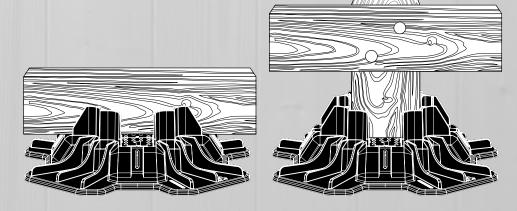
TuffBlocks are not designed for use in structures elevated more than one (1) metre from the ground and should be installed on stable ground (see website for more details). As always, it is recommended to check your local building guidelines before starting any construction - we always suggest you get the thumbs up before starting your project. TuffBlocks are more than just a deck foundation, they are a versatile utility block that can be used for an endless number of applications.
