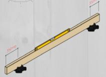
Locate the highest TuffBlock pier. Position a floor joist in or above this first block to your desired height. If the entire deck will be elevated, you will need to have a post in the first TuffBlock.
