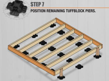
Using the frame as a guide, position the remaining TuffBlock piers directly beneath the frame. The blocks on the perimeter of the deck should be 300mm in from each end.
