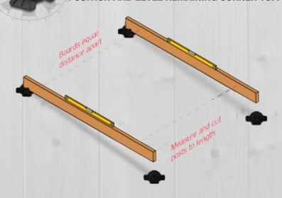
Next, remove the first floor joist closest to the structure. Temporarily position a trim board on top of the first row's post or block, and extend it to the outside corner block. Using a level on top of the trim board, measure the distance from the top of the trim board to the bottom of the pocket on the TuffBlock pier. Cut a post to length. Verify the trim board is level. When level, remove the trim board and repeat for opposite the side.
