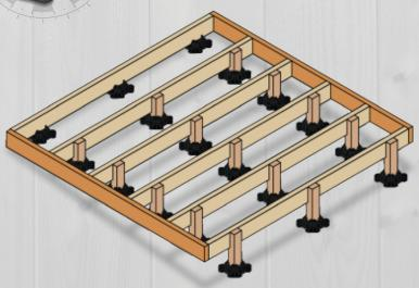
Cut posts to length and position them between the floor joist and the TuffBlock pier. Repeat this step until all posts are cut and positioned. Next, secure all floor joists and posts using two 75mm counter sunk batten screws.
