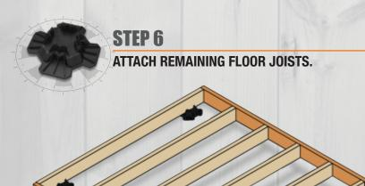
Position and attach the remaining floor joists to the trim boards using two 75mm counter sunk batten screws to attach the floor joist to the trim board.
