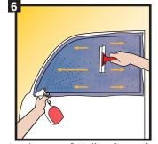
Apply more Solution Spray for lubrication and starting from centre, use Applicator to work out bubbles to edges.
