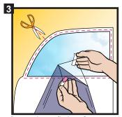
On a clean flat surface, cut film 20mm wider than stencil along all sides. For large curved windows, cut film into strips to avoid wrinkles. Slowly peel away tint backing.
