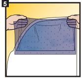
Place adhesive side of film on alass and aently manoeuver into position. Smooth out using hands.
