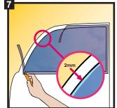
Trim excess tint leaving a 2mm gap for any water residue to escape.
