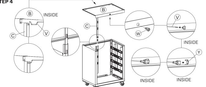
Connect the lock positioning plate (Y) and locking channel (C) to the top panel (B) then slide the top panel (B) down onto the cabinet frame ensuring the locking channel (C) slides smoothly into its slot in the back panel (D). Once the top panel (B) is sitting firmly on the frame, insert the lock (W) through the pre-cut hole and connect the locking tongue (V) and lock positioning plate (Y) to the lock (W).
