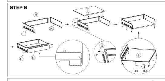
Now that frame is complete construct the three shallow drawers by fixing parts H, I, J, K and L together using the provided 8g x 10mm self tapping screws (U). Ensure the rails on parts J and K are positioned on the outside of each drawer.
