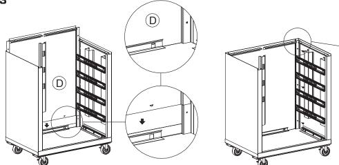
Once the left and right panels are in place fix the back panel (D) to the base before also fixing it to the left and right panels using the provided 8g x 10mm self tapping screws (U).
