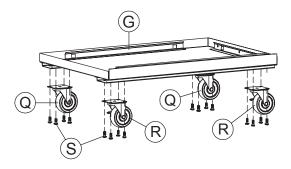
Place the bottom panel (G) upside down on the ground. Fix the castors with brakes (R) to one side of the panel with the provided M8 x 15mm panhead screws (S). Then fix the remaining castors to the other side with screws.
