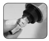
4. Pull back the sleeve on hose fitting, insert male end & release sleeve on hose fitting.
