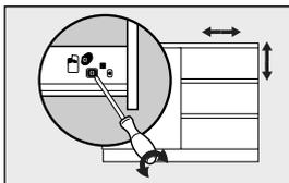
Adjustment point for drawer front alignment if required.
