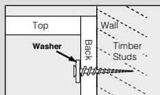
When fixing vanity unit to wall, use washers around the top fixing positions. This will decrease pressure applied to the screw head.
