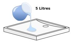
Put base on a level surface and water test with 5 litres of water to ensure it drains correctly. If this is not possible, a small spherical object placed in each corner will suffice.
