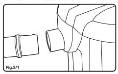
Insert the flexible hose into the inlet on the main body of the vacuum cleaner. Turn the hose clockwise until it cannot be turned any further (Fig.3/1).
