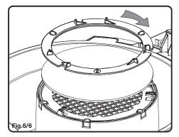
5. Replace with a new filter inside and turn the retaining disc clockwise to secure. (Fig.6/6)
