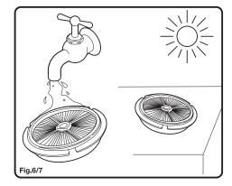
**NOTE:** Do NOT use any detergents or boiling water to wash the filter.
