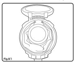
3. The pre-motor filter is found in the centre of the dirt container. Rotate the filter retaining disc anti-clockwise to gain access to the filter (Fig.6/4).
