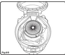
3. The HEPA pre-motor filter is found in the centre of the dirt container. Rotate the filter clockwise to remove (Fig.6/9).
