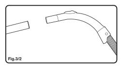
2. Push the extension tube on to the end of the handle. The extension tubes can be used together to lengthen or shortened by using one section of the extension tube as required.(Fig.3/2).
