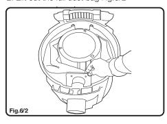
3. Dispose the full dust bag and insert a new dust bag into the vacuum cleaner. Align the front of the dust bag with the air entrance.
