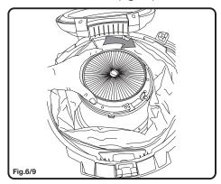
4. Gently tap the filter against the side of the rubbish bin to remove excess dirt. The filter may then be rinsed in cool water. Allow to thoroughly air dry before replacing. Replace the filter every 3-6 months depending on useage or when the filter
