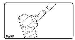
3. Fit the combination floor head by pushing onto the extension tube. (Fig.3/3).
