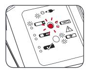
5. The green LED will illuminate once the battery is fully charged.
