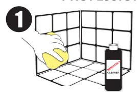
Use **Maxiclean** to clean joint before applying silicone. Joint must be free of any contaminants eg: Dust, Moisture.
