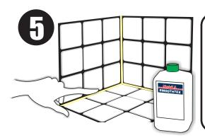
For a final touch-up use your finger, dipped in **Smoothtex** , with minimum pressure to smooth over joint ..
