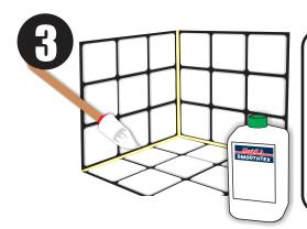
Using the **Smoothtex brush**, with minimum pressure, apply generous amounts of **Smoothtex** leaving the last 5cm free of **Smoothtex**. This allows the next area of silicone to adhere to the last if required.
