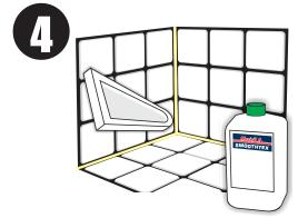
Use the applicator to remove excess silicone and form a smooth and tidy joint. Be sure to frequently dip the applicator in the **Smoothtex**. By holding the applicator at different angles it can be used to remove various amounts of silicone needed to achieve the joint size required. Dispose of excess silicone thoughtfully.
