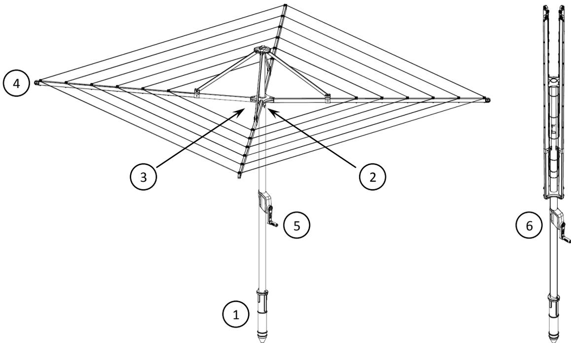
1. 3 adjustable Ground Mount heights, providing up to 150mm of adjustment
