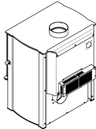
When using the blower, allow the wood fire to reach operating temperature (approximately one hour), before turning it on. The increased airflow from the blower cools the firebox and could affect the start-up combustion efficiency if the blower is turned on too early.
