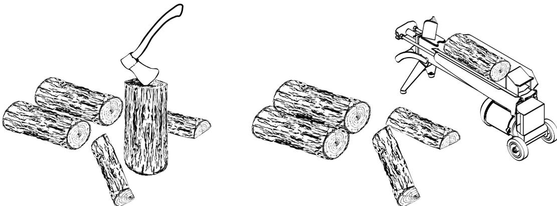
Wood should be split to a range of sizes, from about 75 mm to 150 mm in cross section. Having a range of sizes makes starting and rekindling fires much easier. Often, the firewood purchased from commercial suppliers is not split finely enough for convenient stoking. It is sometimes advisable to resplit the wood before stacking to dry.
