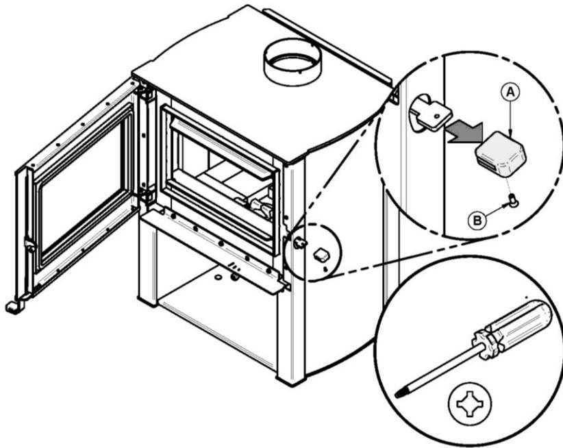
2. Unscrew screw (B) and remove the handle (A).
