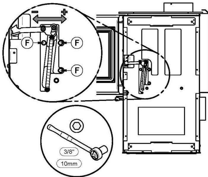
5. To adjust door tightness, slightly loosen the bolts (F). The more distant from the door is the mechanism, the stronger the tightening will be.
