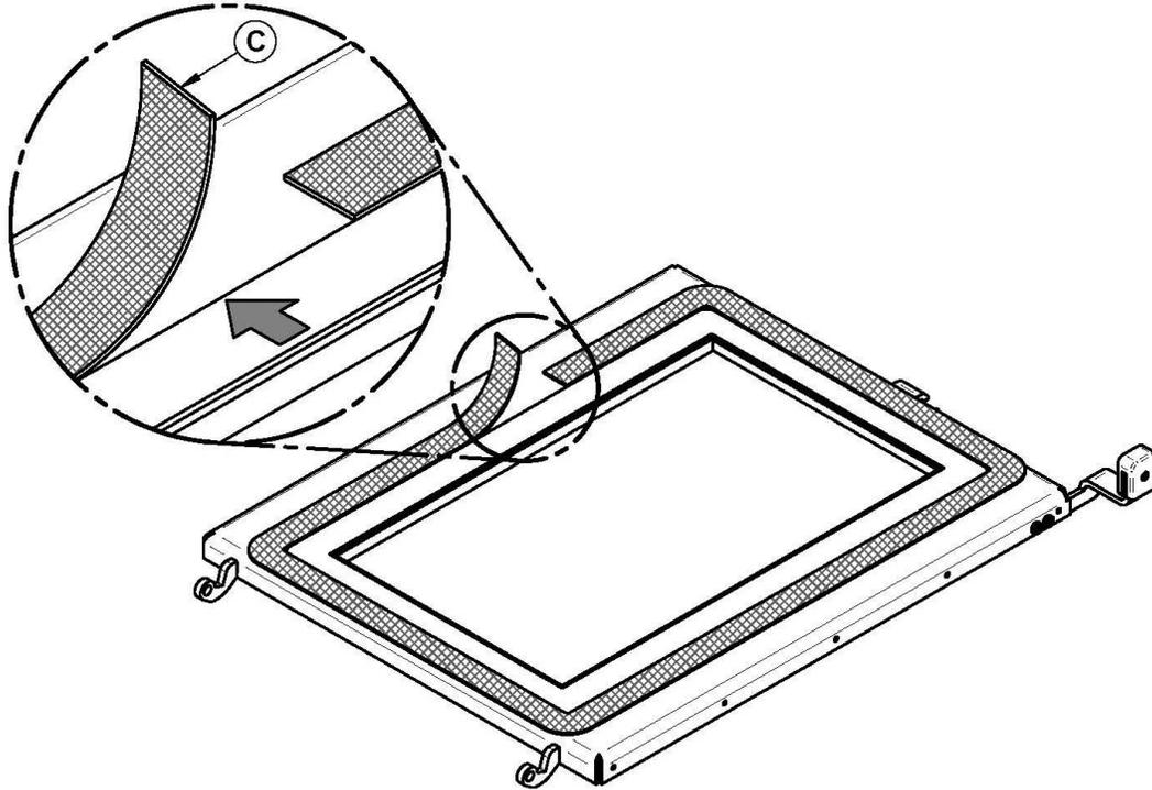
Reinstall the glass, being careful to centre the glass carefully in the door. Do not over-tighten the screws. Note that the two main causes of broken door glass are uneven placement in the door and over-tightening of retaining screws.
