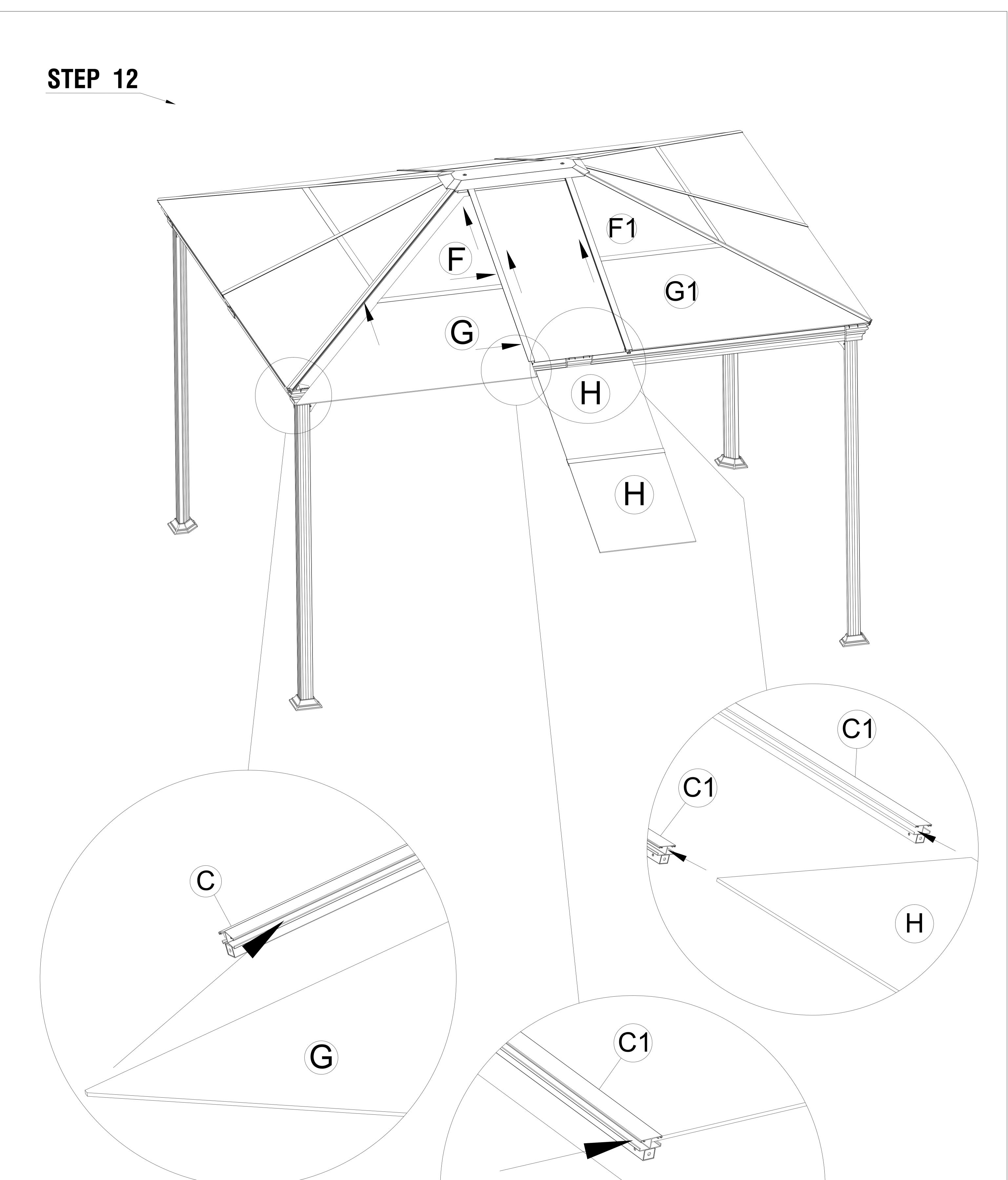
Secure the polycarbonate panel(F)(G)(E) with the four inclined tube(C), the middle inclined tube (C1)
