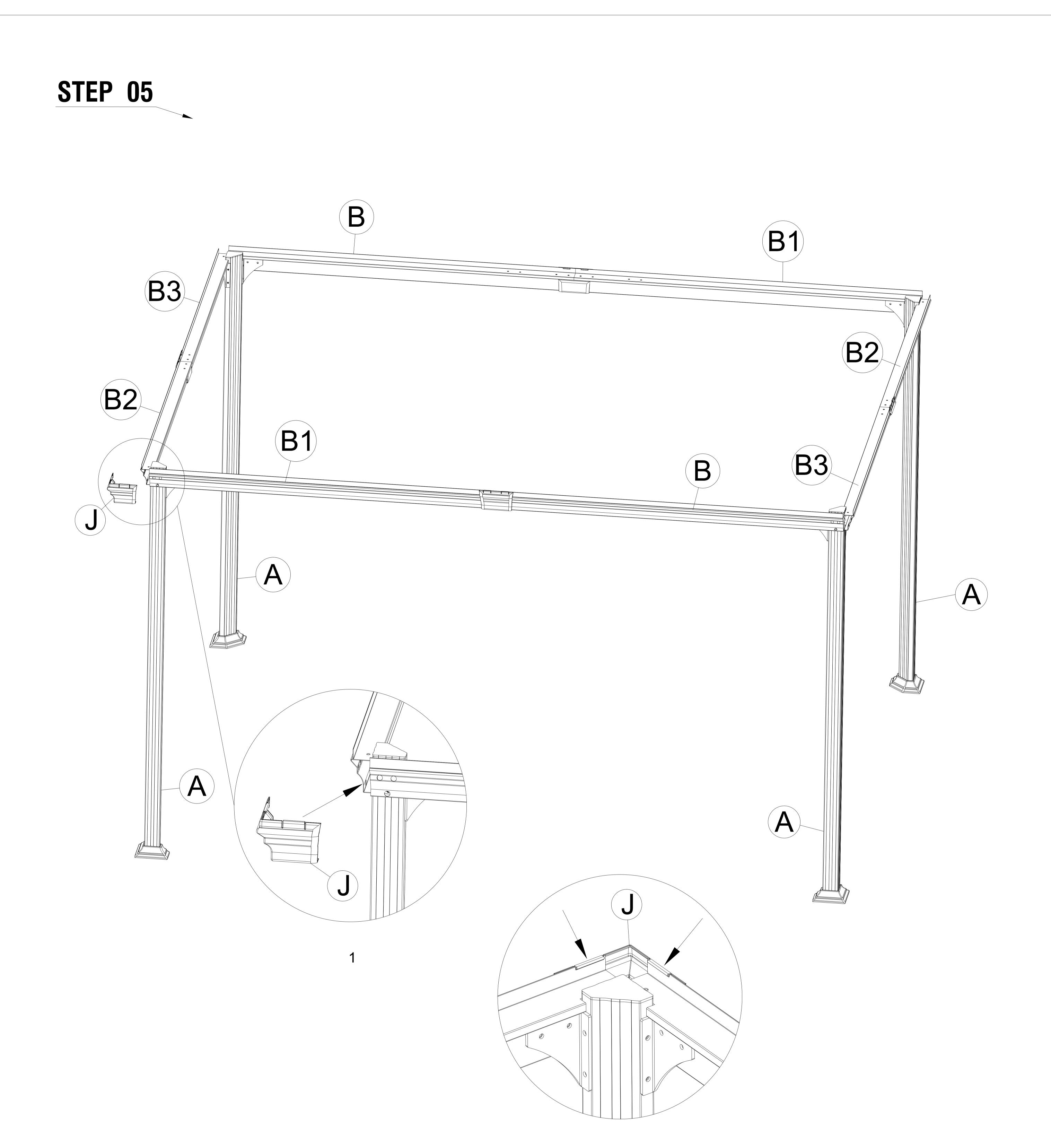
Secure the four package plate(J) with the ring beam (B1) and ring beam (B2), push.
