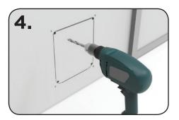
4. Drill holes in each of the inside corners with a minimum of 10mm (3/8") drill bit.
