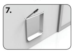
Place outer frame in hole, if the tunnel protrudes through the door, mark around tunnel.
