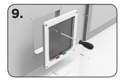
Screw into door from both sides and cover screws with screw covers.
