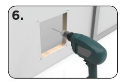
6. Check outer frame fits opening and screw holes align. Drill 3mm pilot holes.
