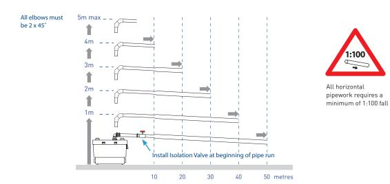
Following vertical lift, increase discharge pipe diameter by one size on the Horizontal run to Sewer or vent connection. **N.B. VERTICAL LIFT MUST PRECEDE HORIZONTAL RUN**
