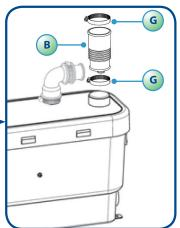
To connect to a lid inlet, cut off the sealed cap with a Stanley knife or hacksaw and connect using the rubber connector (**B**) provided. Tighten with the metal hose clips (**G**).
