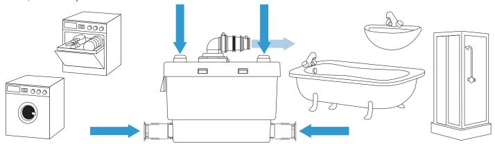
The Sanispeed will activate automatically following the inflow of waste water from any of the above fixtures.
