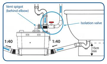
To connect a shower/bath, ensure that the trap exit is at least 15cm above floor level. Although not obligatory, a lid connection may be used to run an external air vent.
