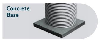
A concrete slab base is the most suitable base for your Aquaplate® rainwater tank. Construction of a concrete base needs a minimum of 100mm thick concrete and F62 mesh, on a flat level area. If the tank is to be positioned in an area that is on a slope then the thickness of the slab is to be increased and the mesh to be a higher grade. The slab must be flat, smooth and level. Finish with a metal trowel is advisable.
