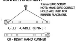
PLACE YOUR RUNNERS INTO THE DESIGNATED HOLES MAKING SURE THE WHEEL IS FACING TO THE FRONT OF THE GABLE. HOLE POSITION NO 1, 8 AND 15.
