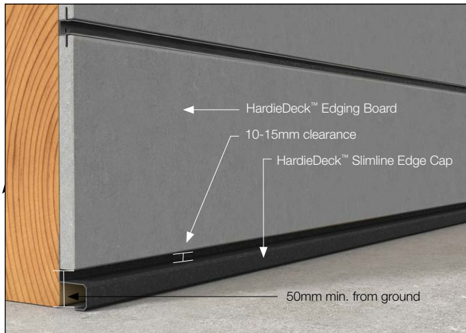
FIGURE 12 BOTTOM FINISHING DETAIL AND CLEARANCE
