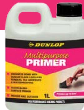
DUNLOP PRIMER is a water-based primer which enhances the bond between substrates and DUNLOP FLOOR LEVELLERS, RENDERS, TILE ADHESIVES and WATERPROOFING products. Suitable substrates include new and old concrete, particleboard, marine plywood and fibre-cement sheets. DUNLOP PRIMER is suitable for indoor and outdoor projects over walls and floors.
