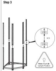
Join the upper and lower legs with the connector pins, as shown in the diagram, taking into account upright position. Note: The legs are designed to sit directly on top of each other – don't overlap them. Handy Hint: Flathead screwdriver may be used to tap in connector pins.
