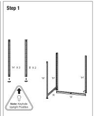
Place foot end caps onto the bottom of the 5 legs 'H' and 'l'. Note upright position. Place shelving bracket 'A' onto the legs. A rubber mallet can be used to lightly tap all brackets into the keyholes of the legs into place. Allow one keyhole free between the foot cap and the shelving bracket.
