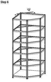
Apply remaining brackets as above to desired height. Ensure that brace 'G' are fixed to all shelves.
