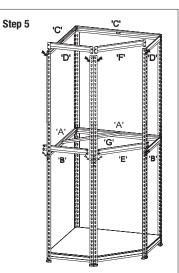
Fix brackets 'A' so that the top rivet sits on the upper legs and the bottom rivets sit on the lower legs. Repeat with brackets 'B' and 'E', followed by brace 'G' as done previously. Fix brackets 'C', 'D' and 'F' at the very top allowing room for the MDF board to sit flush against the legs. Repeat as per previous step.
