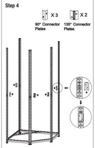
Gently tap in 90° connector plates into rear and side upright joints, repeat process with 135° connector plates in front two upright joints.
