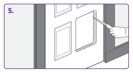
Using a reciprocating jigsaw, cut out the opening, cutting along the pencil outline.
