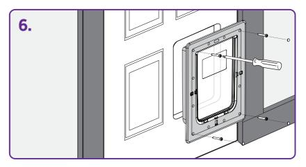
Place both frames into the opening and secure with screws and caps provided.
