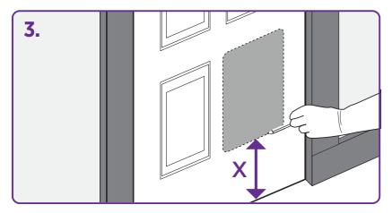
Cut out template supplied in box, line up bottom of cut out with height (x) and trace onto door.
