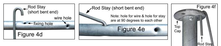
**5.** Wire holes on the Arms need to be horizontal and may need adjusting. To do this, insert a screwdriver through a pair of wiring holes and use it as a lever to rotate the Arm until horizontal. Repeat on other Arms.
