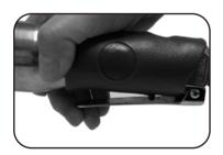
Select the direction of rotation by turning the forward/reverse lever anti-clockwise for forward or clockwise reverse rotation.
