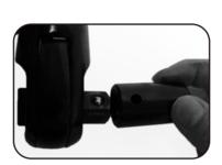
Note: The air ratchet should only be used with impact sockets. Standard sockets may shatter and break.
