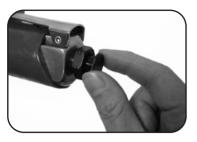
4. Pull back the sleeve on hose fitting, insert male ratchet end & release sleeve on hose fitting.
