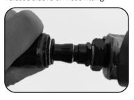
2. Wrap the threaded male end with teflon tape in a clockwise direction.
