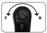
3. After each use, place one drop of oil into the ratchet, through the air inlet.
