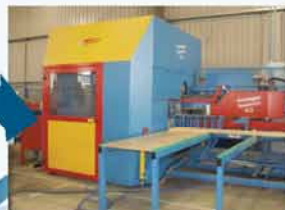
Automated CuttingSystem (includes precutting web penetrations)
