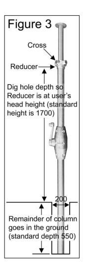
**3a.** Hoists with Plastic Handle Casing (Elite, Deluxe & Special): Remove the column from the hole and insert the Steel Rod through the pre-drilled holes in the bottom of the column. Place column back in the hole. Other models do not require Steel Rod, they have pressed ends to hold firm in the concrete.
