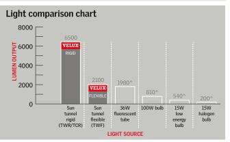
Light transmittance of VELUX Sun Tunnels depends on parameters such as sky conditions (cloudy/sunny), direction of sunlight, orientation and length of Sun Tunnel. VELUX Sun Tunnels in this chart have been tested with a 1 metre shaft, on a 15° roof pitch in summer, at noon on a sunny day using a photometer. (TWR rigid tunnel emits 440 lumens when measured on a cloudy winter's day).
