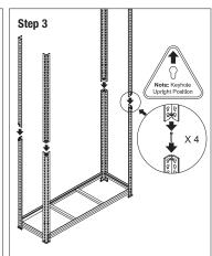
Place MDF board on bottom shelf to minimise buckling. Join the upper legs to the lower legs with the connector pins. Note: The legs are designed to sit directly on top of each other – don't overlap them. Handy Hint: Flathead screwdriver may be used to tap in connector pins.
