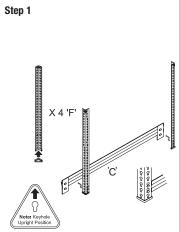
Place foot end caps onto the bottom of the legs 'F'. Note upright position. Place shelving bracket 'C' onto the legs 'F'. A rubber mallet can be used to lightly tap all brackets into the keyholes of the legs into place. Allow one keyhole free between the foot cap and the shelving bracket.
