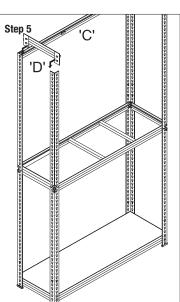
Fix brackets 'C' at the very top allowing room for the MDF board to sit flush against the legs. Repeat with brackets 'D'.
