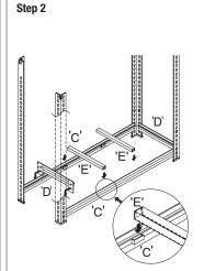
Use shelf bracket 'D' for the side brackets using the shelf bracket from Step 1 as a guide for height. Allow 1 keyhole free from the ground as shown in the diagram. Use same shelving brackets for opposing sides as shown in the diagram. Place braces 'E' as shown.
