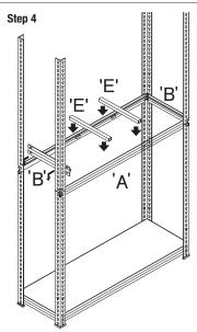
Fix brackets 'B' so that the top rivet sits on the upper legs and the bottom rivets sit on the lower legs. Repeat with brackets 'A', followed by braces 'E' as shown.
